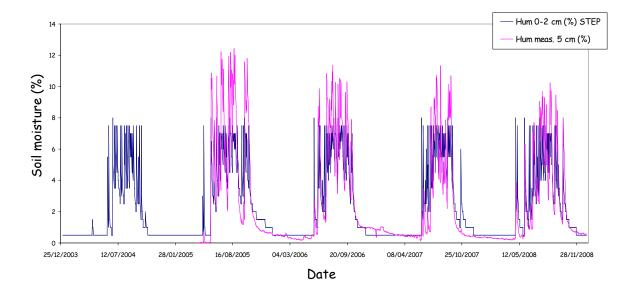
Fig. 2. Soil moisture calculated by STEP at the surface layer (0-2cm) in blue, mean soil moisture measured at 5cm in pink, for years 2004 to 2008 at Agoufou.
