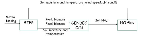
Schematic representation of NO flux modeling coupled to STEP-GENDEC
