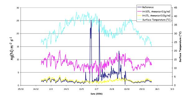
**Fig. 8.** Sensitivity test. In dark blue: reference NO flux in kg(N)ha<sup>-1</sup>yr<sup>-1</sup>, in yellow: NO flux with H=2% and mineral N=0.01gm<sup>-2</sup>, in pink: NO flux with H=10% and mineral N=0.1gm<sup>-2</sup>, in light blue: surface temperature in  $^{\circ}$ C, for year 2006.
