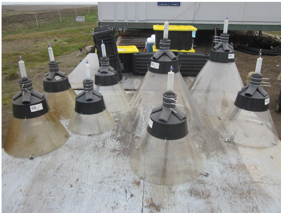
Figure A1. Picture of the homemade funnels deployed in ponds and lakes (photo taken in July 2014 just after their removal).
