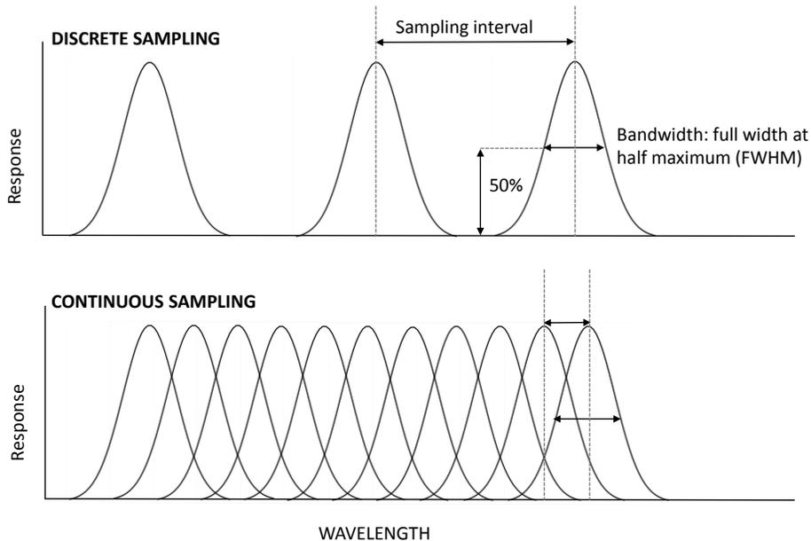
**Figure 2.** Different sampling strategies: discrete vs. continuous. Spectra resolution denoted by bandwidth and sampling intervals. The narrower the bandwidth and the shorter the interval between bands the higher will be the resolution at which spectral features can be resolved. Note that sensor responses are here represented as Gaussian just for simplicity reasons but typical sensor responses may present different shapes.
