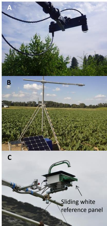
**Figure 5.** Hyperspectral systems developed during EUROSPEC. The Piccolo system **(a)** and the SIF-Sys **(b)** use a single spectrometer to measure two fields of view by means of a bifurcated fibre optics. The White-Ref system **(c)** uses a sliding white reference panel to measure irradiance. See further details in the text.
