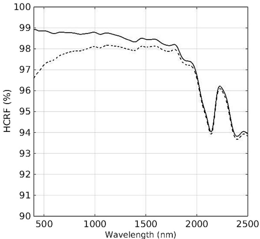
**Figure 3.** Spectralon<sup>®</sup> panel reflectance before (dotted line) and after cleaning (solid line). The panel had been “lightly” and carefully used in the field for one season. Data provided by C. MacLellan, NERC/NCEO Field Spectroscopy Facility, GeoScience, U. of Edinburgh.
