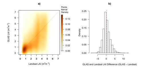
**Figure 4.** Comparison between Landsat LAI and GLAS LAI over contiguous US: **(a)** density scatter plot of Landsat and GLAS LAI ( $r^2 = 0.18$ , bias = 0.18 and RMSE = 2.02); **(b)** Difference between Landsat and GLAS LAI. Darker kernel density color refers to more clustered distribution of LAI pairs.
