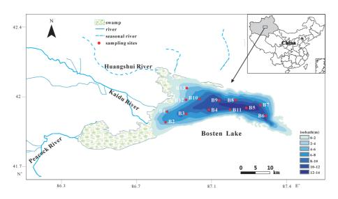
**Figure 1.** Map of the Bosten Lake with the water depth and the 13 sampling stations (red dotes). Bathymetric was measured in 2008 by Wu et al. (2013) and bathymetric contours were plotted by using software ArcGIS 9.3 and Corel DRAW X3.
