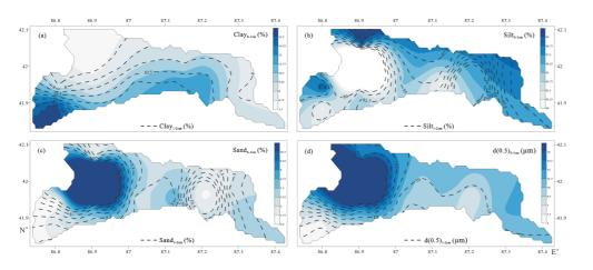
**Figure 2.** Distributions of **(a)** clay, **(b)** silt, **(c)** sand and **(d)** the median diameter (d(0.5),  $\mu$ m) in the 0–1 cm (color map) and 1–2 cm (dashed lines). The spatial distribution maps (Figs. 2–7) were produced using Surfer 9.0 (Golden Software Inc.) and the interpolated data in the maps was made using the Kriging method of gridding.
