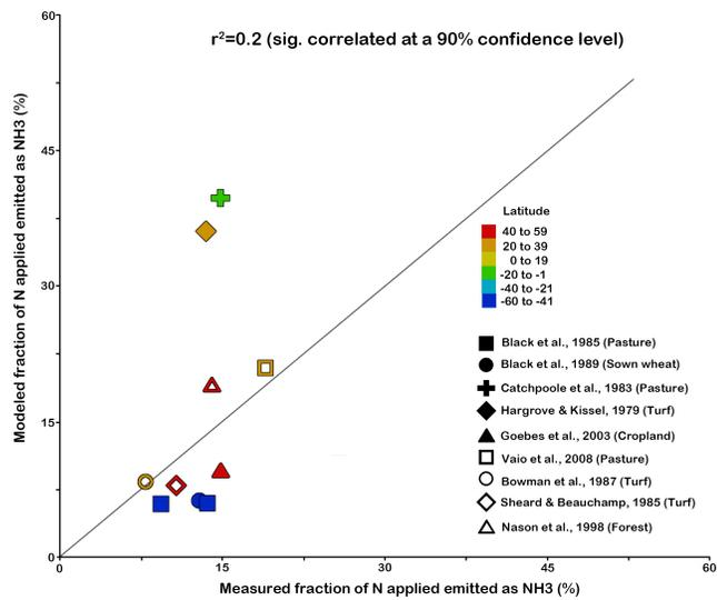
Figure 3. Comparison of model to measurements for percentage of nitrogen lost as NH<sub>3</sub> emissions from fertilizer (see supplementary Table 2). Symbol color gives the latitude at which the measurement was made; symbol shape gives the study and type of fertilizer application.
