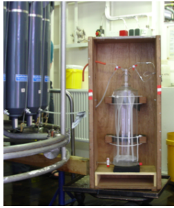
Figure 2: Experimental setup for headspace sampling, a) sampling of the surface water into the glass vessel, connected to the Niskin bottle rosette, b) scheme of the experimental setup
