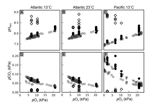
Fig.2: pH<sub>NBS</sub> and pCO<sub>2</sub> in incubation water (black symbols), compared to environmental levels (grey symbols) for the ETNA OMZ and the ETSP OMZ. Black circles: CO<sub>2</sub>-plus
