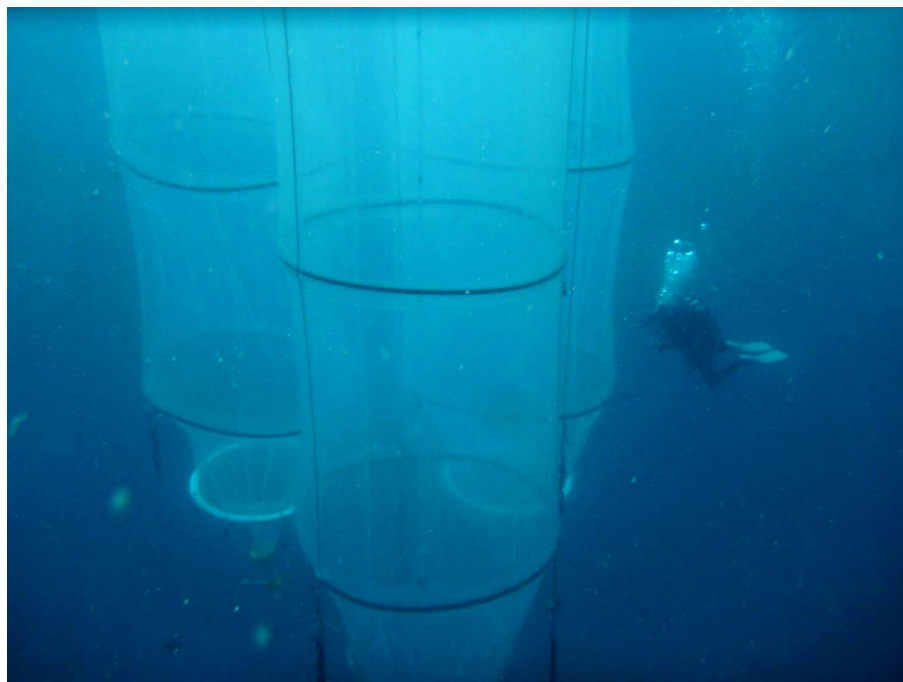
Figure 2. Picture of the VAHINE mesocosms deployed at the exit of the New Caledonian coral lagoon.
