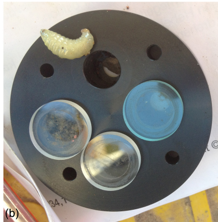
Figure 4. Skye multi-spectral sensors showing (a) mud wasps, and (b) wasp larvae in sensor tubes.
