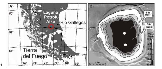
Figure 1. Map of Southern Argentina displaying the location (**A**) and bathymetric map (**B**) of Laguna Potrok Aike showing the two drilling sites (Zolitschka et al., 2006). Pore water and geomicrobiological samples were retrieved from cores at site 5022-1, whereas sediments for pigment analysis were obtained from cores at site 5022-2.
