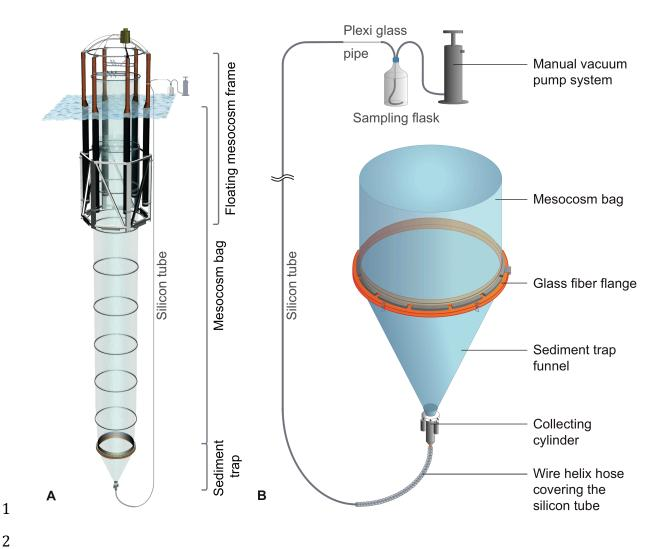
**Figure 1. (A)** Technical drawing of the KOSMOS flotation frame with unfolded TPU enclosure bag and attached funnel-shaped sediment trap. **(B)** A silicon tube connects the collecting cylinder at the tip of the sediment trap with a 5 L sampling flask. A wire-reinforced hose prevents current related bending of the first 1.5 meters. Particles can be easily detected in the Plexiglass® pipe linking up the silicon tube with the sampling flask.
