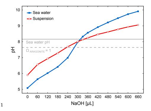
**Figure 4.** Titration of 500 mL sea water (blue, filled box and line) and 500 mL particle suspension (red, empty box and line) with 3 M NaOH after addition of 150  $\mu$ L 2.4 M FeCl<sub>3</sub> solution. The grey solid line indicates the pH of seawater before any manipulation. pH (NBS scale) was measured at 25°C with a stationary pH meter (713, METROHM). Calculated aragonite saturation state of  $\Omega = 1$  is represented by the grey dashed line.
