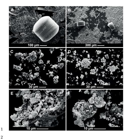
Figure 6. Scanning electron microscopy (SEM) photographs of two sediment trap samples before (A, B) and after grinding (C – F). (C) and (D) represent the average grain size of the ground samples, while (E) and (F) reveal details visible at 2500 fold magnification.
