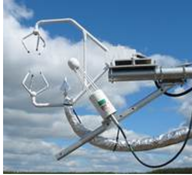
Figure 1: Tilted open-path and inlet for closed-path system at the HJP02 Fluxnet Canada site (Photo by Zoran Nesic, UBC)
