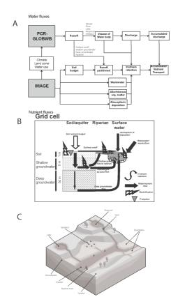
**Figure 1. (a)** Scheme of the model framework with PCR-GLOBWB and IMAGE and the data flows between the models; **(b)** scheme of the flows of water and nutrients, and retention processes within a grid cell; **(c)** scheme of the routing of water (with N and P) in a landscape with streams, rivers, lakes, wetlands and reservoirs; each type of water body within a grid cell is defined by an inflow or discharge, depth and area. Floodplains may be temporarily flooded.
