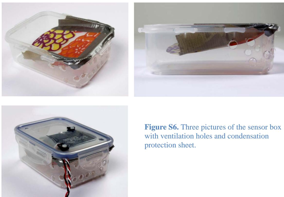
**Figure S6.** Three pictures of the sensor box with ventilation holes and condensation protection sheet.
