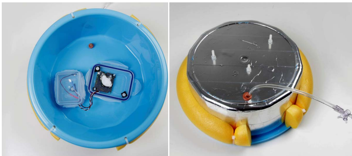
Figure S5. Inside (left) and outside (right) of the chamber type used. The tube with the 3-way syringe valve to the right is for manual sampling at the end of selected deployments to check sensor performance.
