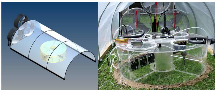
Figure 1. The nested wind tunnel system. Note high speed fans within the toroid at East and West compass points, with anemometers measuring wind speeds at points North and South. Toroid vents are open at this point and all internal fans are off. Wind tunnel sides are PAR transparent in this picture and drum fans at the end of the agricultural tunnel are off. Pressure differential gauges can be seen above fan banks and the PAR sensor is front and center on the top of the flux chamber.
