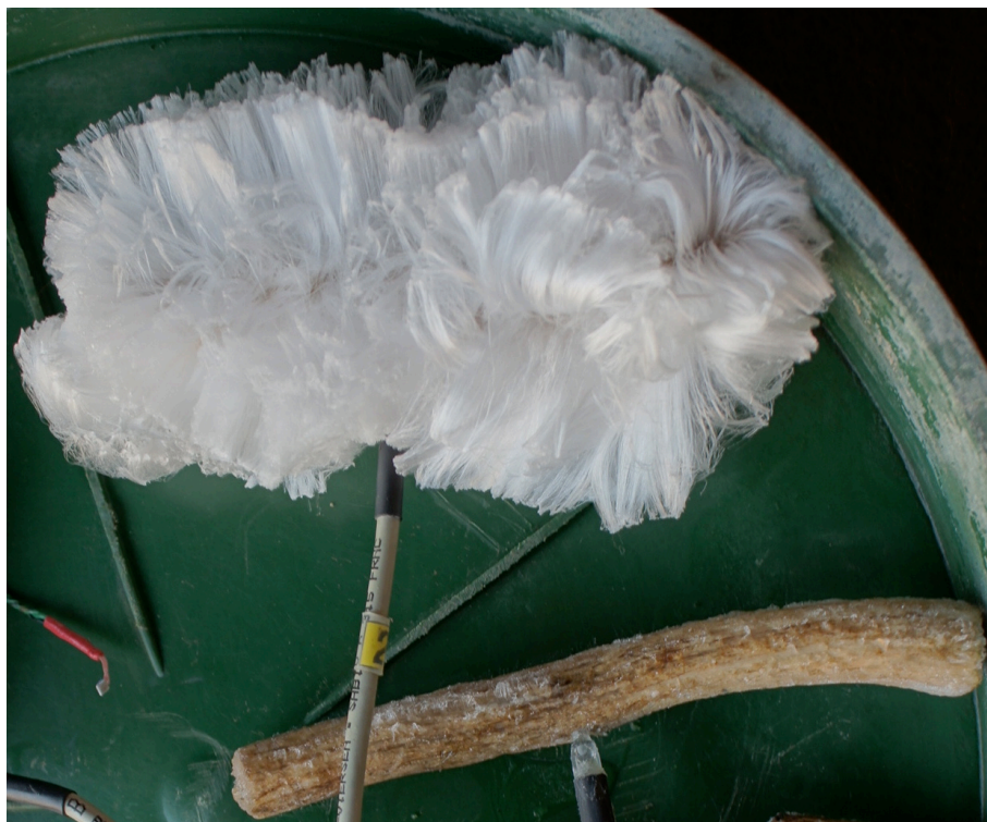
Figure 10. Situation in the morning of 15 January 2012: heat-treated piece (1, bottom right), piece (2, top) with abundant hair ice, air temperature sensor (3, bottom left) with red insulation.
