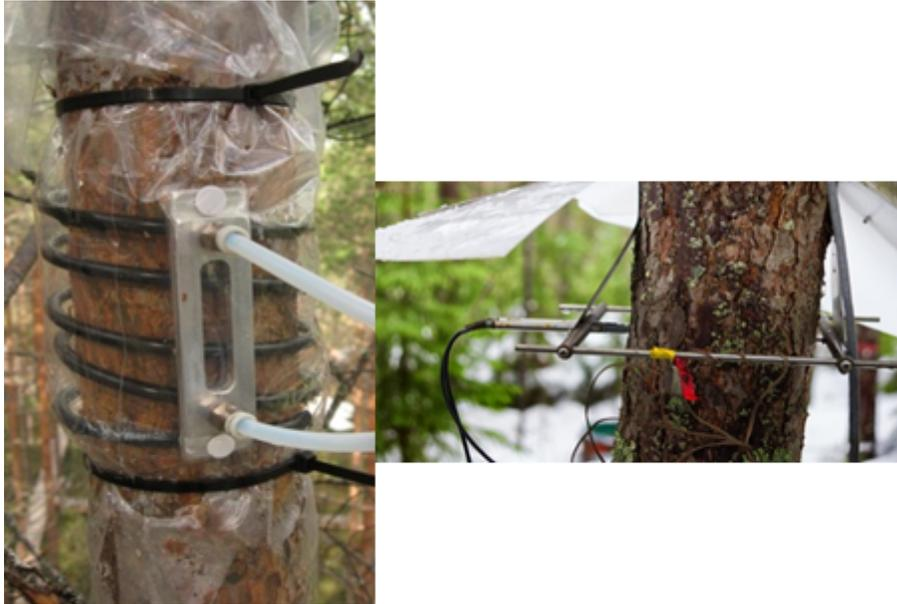
**Figure 2.** The stem enclosure around a Scots pine stem at a height of 12 m (left) and a linear variable displacement transducer to measure stem radius changes (right).
