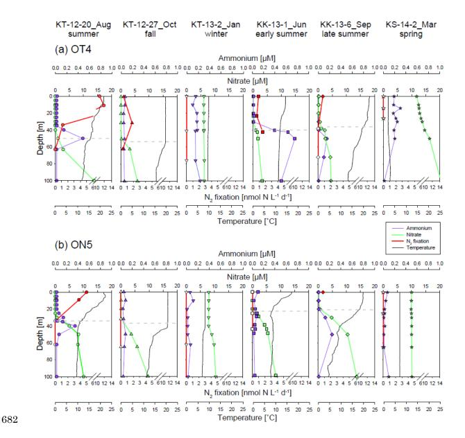
Fig. 5. Time-series variations in the vertical profiles of temperature [°C] (black), ammonium (purple) and nitrate (green) concentration [μM], and nitrogen fixation (red) [nmol N L<sup>-1</sup> d<sup>-1</sup>] at Stns (a) OT4 and (b) ON5. Open symbols indicate that nitrogen fixation was not detected. The horizontal dashed line indicates the nitracline depth. The strait lines of temperature and nitrate were ascribable to strong mixing.
