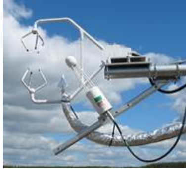
Figure 1: Tilted open-path and inlet for closed-path system at the HJP02 Fluxnet Canada site (Photo by Zoran Nestic, UBC)
