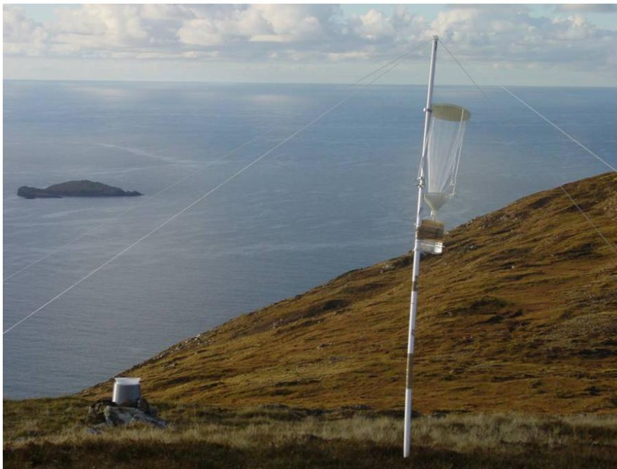
**Fig. 1.** Cloud collector set up on Caepabhal. Collector was erected onto the end of a 2 m pole and secured with guy ropes.
