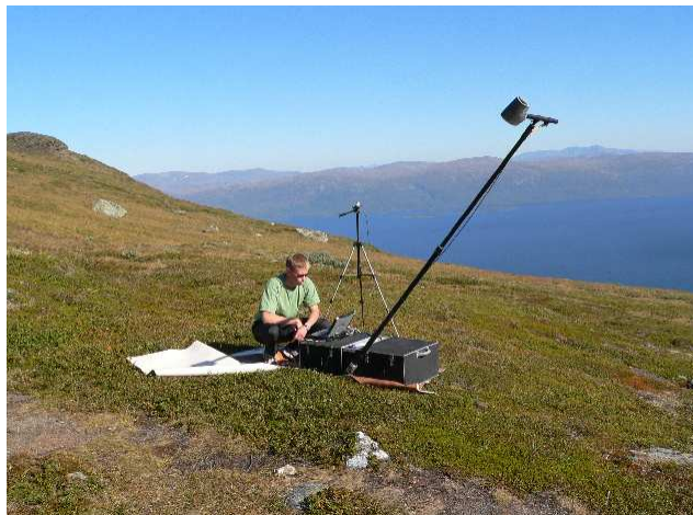
Fig. 2. Figifigo measuring BRF in Abisko, Sweden.
