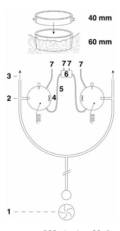
Fig. 1. Twin-cuvette system to measure BSC-related net CO<sub>2</sub> flux: (1) radial fan on 25.4-mm Teflon tubing, (2) 25.4-mm to 12.7-mm Teflon connection to cuvette, (3) 25.4-mm open end tubes, (4) cuvette fan, (5) 6.4-mm connection, (6) infrared gas analyzer, (7) flow control and pumps. Cuvette top height 40 mm, collar height 60 mm, both ID 143 mm; transparent Teflon cuvette window on top 0.016 m<sup>2</sup>. 1994
