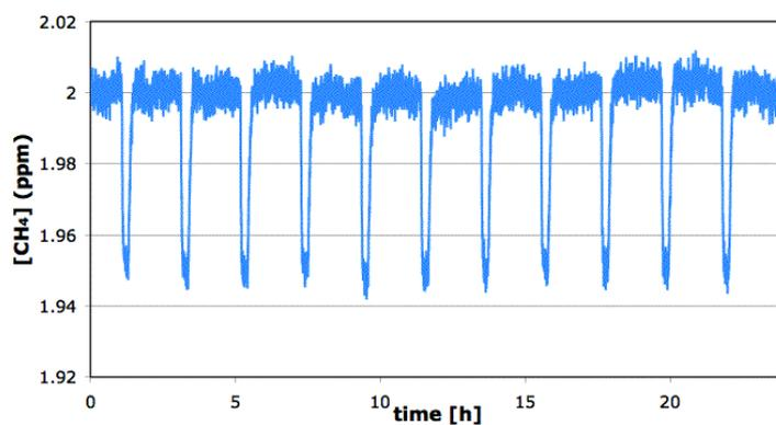
**Fig. 5.** Typical 24 h snapshot of raw CH<sub>4</sub> concentration data from the optical instrument during the long time UV irradiation experiment. During each 2 h period the UV lamp is switched on for 105 min and off for 15 min to monitor possible instrument drift and to continuously verify that the CH<sub>4</sub> emission signal is related to UV irradiation. All other conditions stay constant.
