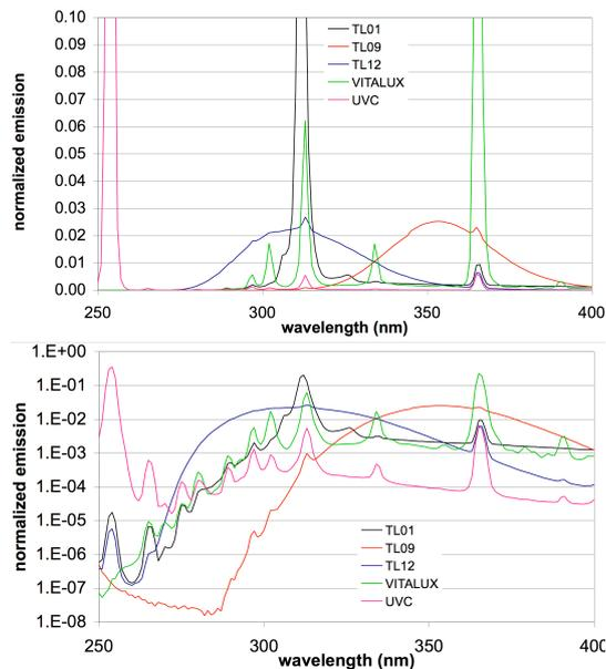
**Fig. A1.** UV spectra of the light sources employed in our study, obtained with a calibrated standard UV-visible spectroradiometer (model 752, Optronic Laboratories Inc., USA). Top, linear scale, bottom, logarithmic scale. The spectra are normalized to yield the same total (250–400 nm) UV emission.
