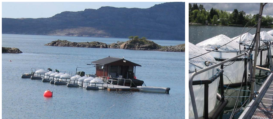
Fig. 1. PeECE III experimental set-up at Large-Scale Mesocosm Facility of the University of Bergen in Espesrend, Norway. Left: array of 9 mesocosms in front of the floating raft. Right: Mesocosm enclosures were covered by gas-tight tents made of ETFE (ethylene tetrafluoroethylene) foil, which allowed for 95% light transmission of the complete spectrum of sunlight, including UVA and UVB.
