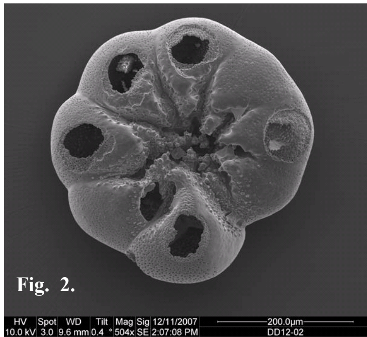
Fig. 2. Scanning electron microscope image of laser ablation craters in Ammonia tepida .
