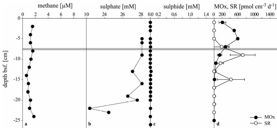
**Fig. 3.** Concentration profiles of (a) methane, (b) sulphate, (c) sulphide as well as rates of aerobic methane oxidation (MOx) and sulphate reduction (SR) in sediments of MUC-core 709-3, which was launched directly above a clam patch (see Fig. 1c for position). Concentrations of ethane were below detection limit. The oxygen penetration depth (grey line) was assumed with 8 cm bsf according to the beige sediment colour of this layer.
