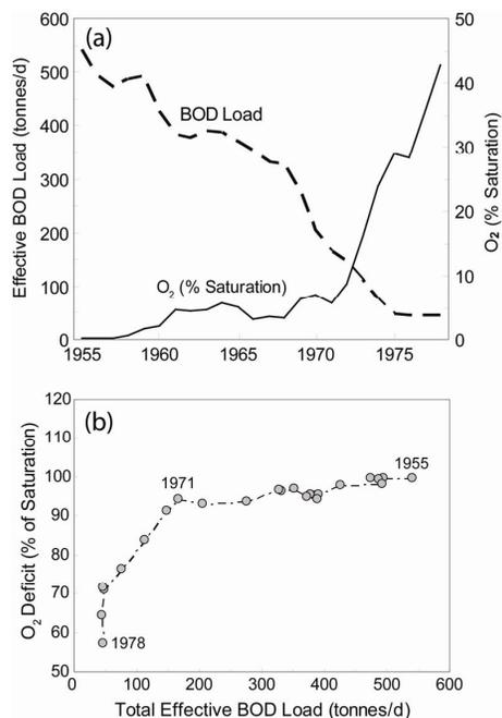
**Fig. 3.** Time series (1955–1980) observations in the upper Thames River estuary (England) for **(a)** BOD load from major sewage treatment plants and summer O<sub>2</sub> % saturation and **(b)** relationship of O<sub>2</sub> % saturation deficit (concentration units below mean saturation) to BOD load showing threshold response of O<sub>2</sub> to reduced BOD load. Data sources referenced within text.
