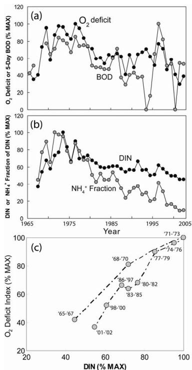
**Fig. 4.** Time series (1965–2002) observations in the Scheldt estuary (Netherlands) for **(a)** BOD and O<sub>2</sub> % saturation deficit, and for **(b)** DIN concentrations and fraction as NH<sub>4</sub><sup>+</sup> and **(c)** relationship of O<sub>2</sub> deficit index to DIN concentration, showing a favorable linear shifting baseline response of O<sub>2</sub> to reduced DIN and BOD loads. Data sources referenced within text.
