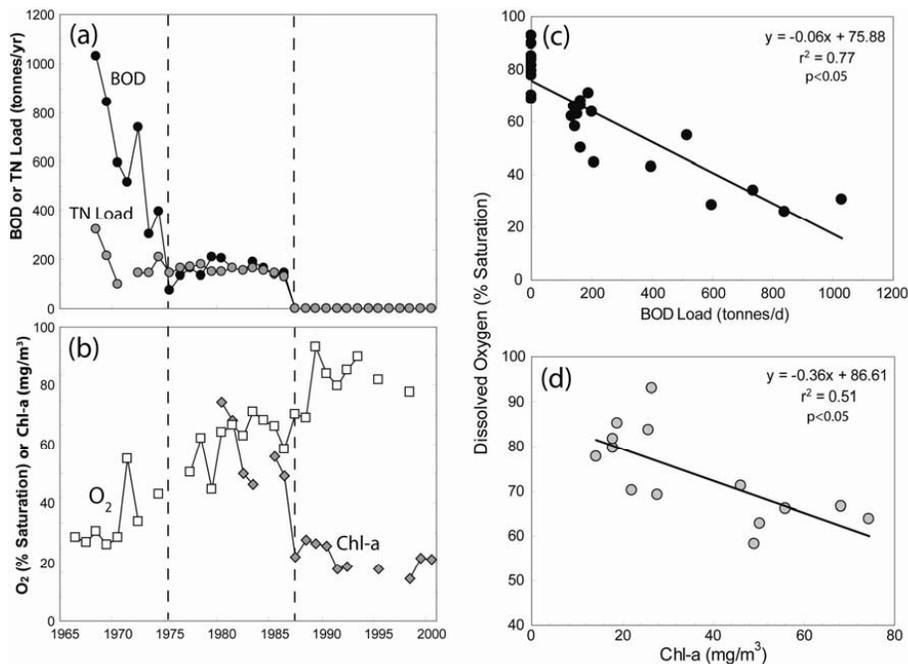
**Fig. 5.** Time series (1965–2000) observations in Laajalahti Bay (Finland) of **(a)** BOD and TN loads and of **(b)** O<sub>2</sub> % saturation and chlorophyll-a. Relationship of **(c)** O<sub>2</sub> % saturation to BOD Load and **(d)** O<sub>2</sub> % saturation to chlorophyll-a. Data sources referenced within text.
