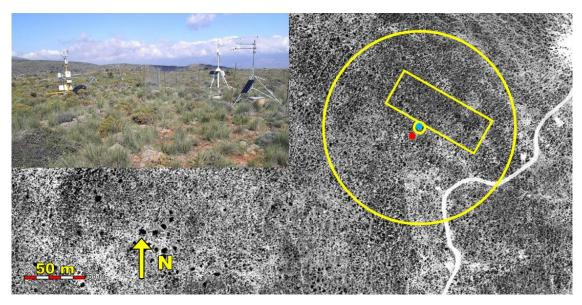
Page 10929, figure's caption has changed to: "**Fig. 1**. Ortoimage of the measuring site, and the position of the two EC (EC<sub>1</sub>: red point; EC<sub>2</sub>: blue point). The rectangular area measured with the GPR, and the boundaries of the source area of EC<sub>2</sub> obtained with the footprint analysis (see Fig. 5 - unstable conditions) are shown. A picture of the site where both EC can be seen is shown on the upper left corner of the figure."
