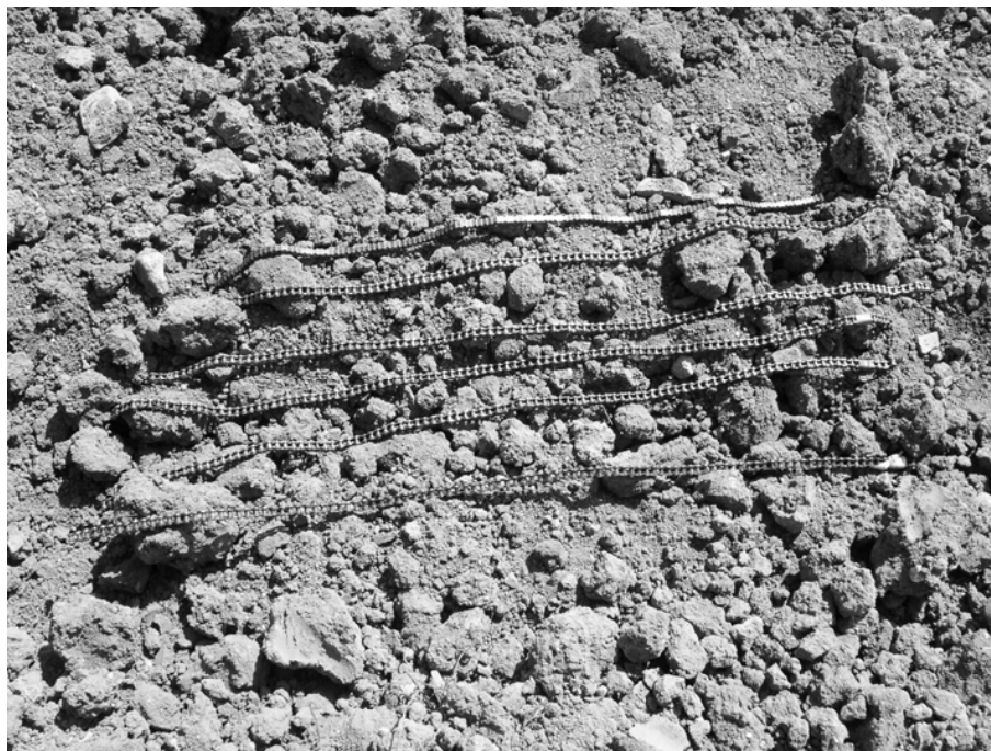
Fig. 4. Chain set used to measure soil surface roughness on soil that has been tilled with a chisel.
