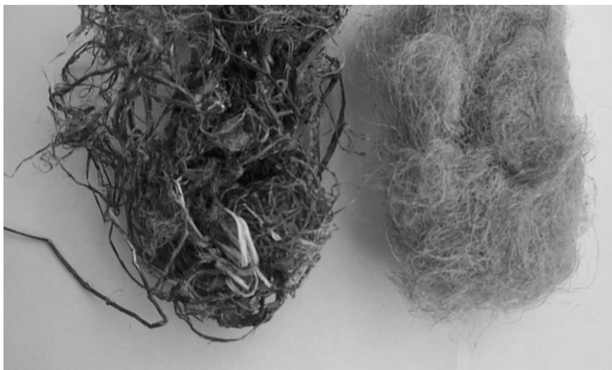
Fig. 4. Broom shoots (left); raw fibers extracted (right).
