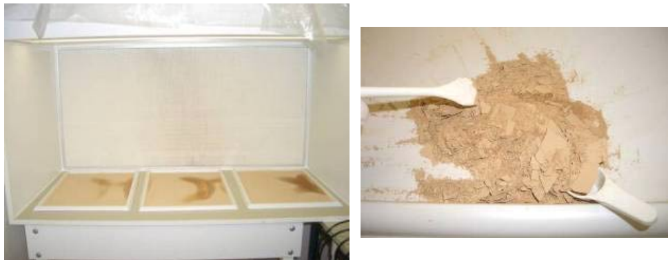
Fig. 6. Artificial aging of the atmospheric particles. The principle is to quickly evaporate a water-aerosol mixing in the typical proportions of a cloud drop that is deposited on ultraclean polypropylene plates under clean air within a laminar flow bench. Water is amended with substances normally observed in Mediterranean marine atmosphere. The added aerosols are the fine fraction of the dust collected in Tunisia. The evaporation leads to a pH gradient in the system induced by proton concentration related to decrease in water volume, exactly as it occurs inside a cloud. (photo S. Tran).
