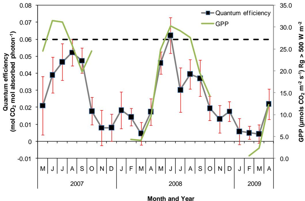
**Fig. 8.** Variation of quantum efficiency and GPP under high light (solar radiation >500 W m<sup>-2</sup>), calculated from monthly data (theoretical maximum quantum efficiency is also shown).
