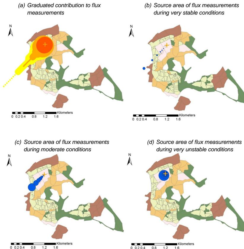
**Fig. B1.** Estimates of flux tower footprint. Colours in the graduated contribution to flux measurements (a, top left) represent atmospheric stability, whereby red = very unstable ( $ZL = -0.5$  m), orange = moderate ( $ZL = -0.1$  m) and yellow = very stable conditions ( $ZL = -0.001$  m).  $ZL$  = flux measurement height/Monin-Obukhov length (based on Schmid and Oke, 1990). Flux tower shown as cross and woodland type types as shown in Fig. 1.
