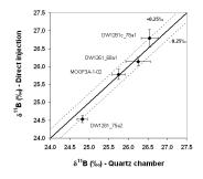
Fig. 1. Comparison of MC-ICPMS analyses using direct injection (d-DIHEN) and conventional introduction for Porites
