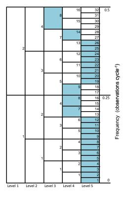
Fig. 5. The 'best bases' for wheat biomass. The nominal partition of the frequency interval by the MODWPT to level 5 is shown with the best bases indicated by the shading. Packet associated with filter  $\mathbf{u}_{k,m}$  is identified by level number k on the bottom of the grid, and packet number m in the cell.
