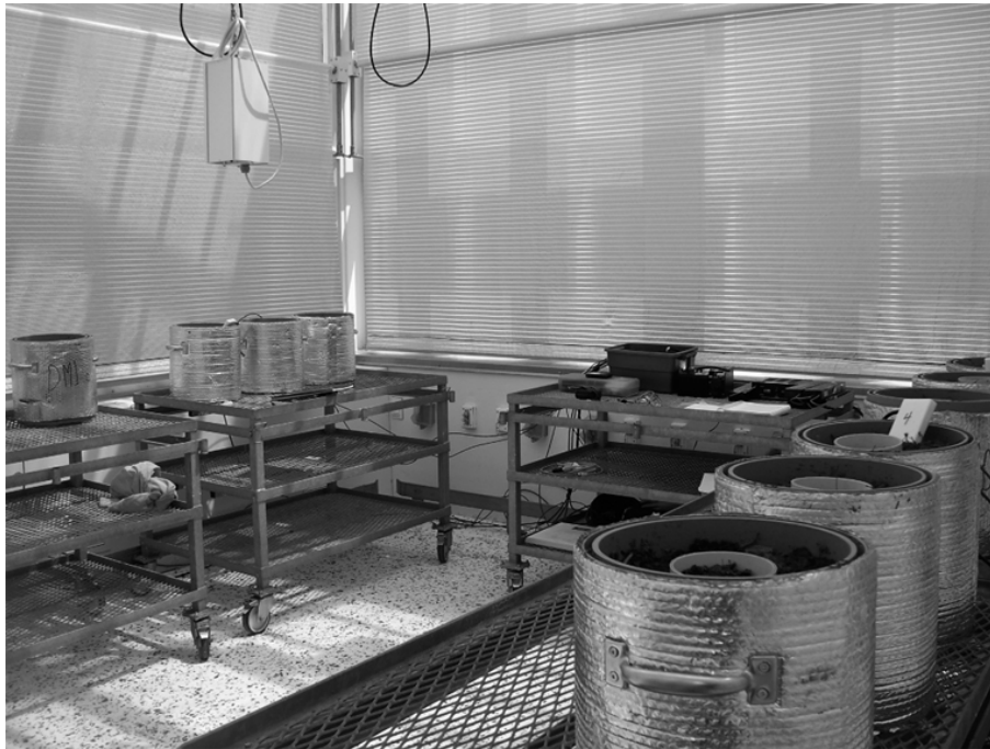
Fig. 1. Experimental set-up in one chamber at the Phytotron facility. Soil microcosms were placed in on trolleys in the climate chamber in triplicate groups that represent the four moisture treatment groups.
