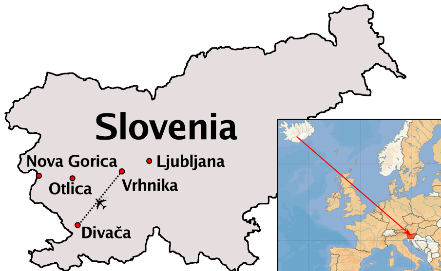
Fig. 1. Map of Slovenia indicating the measuring locations of the campaign. At Nova Gorica and Otlica lidar-based remote sensing was performed. Ground-based in-situ measurements were done in Ljubljana and airborne in-situ measurements were performed during the aircraft ascent at Divača, descent at Vrhnika and during the flight from Divača to Vrhnika and back (dashed line). The inlayed map of Europe indicates the position of Slovenia and Iceland.
