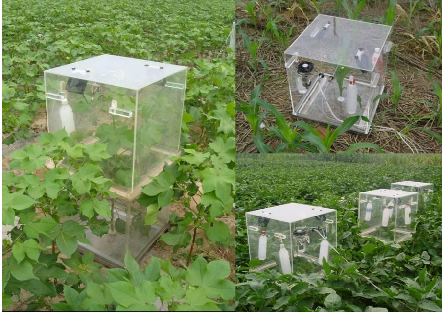
Fig. 2. Photos of measurements using transparent plant chambers in cotton (left), maize (up right) and soybean (down right) fields.
