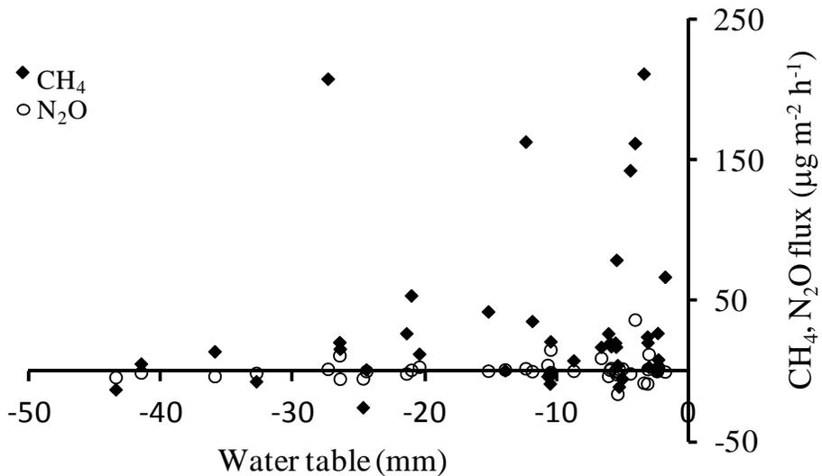
**Fig. 3.** The influence of water table height on CH<sub>4</sub> and N<sub>2</sub>O fluxes at Auchencorth Moss observed during 2007–2010 (data are monthly averages).
