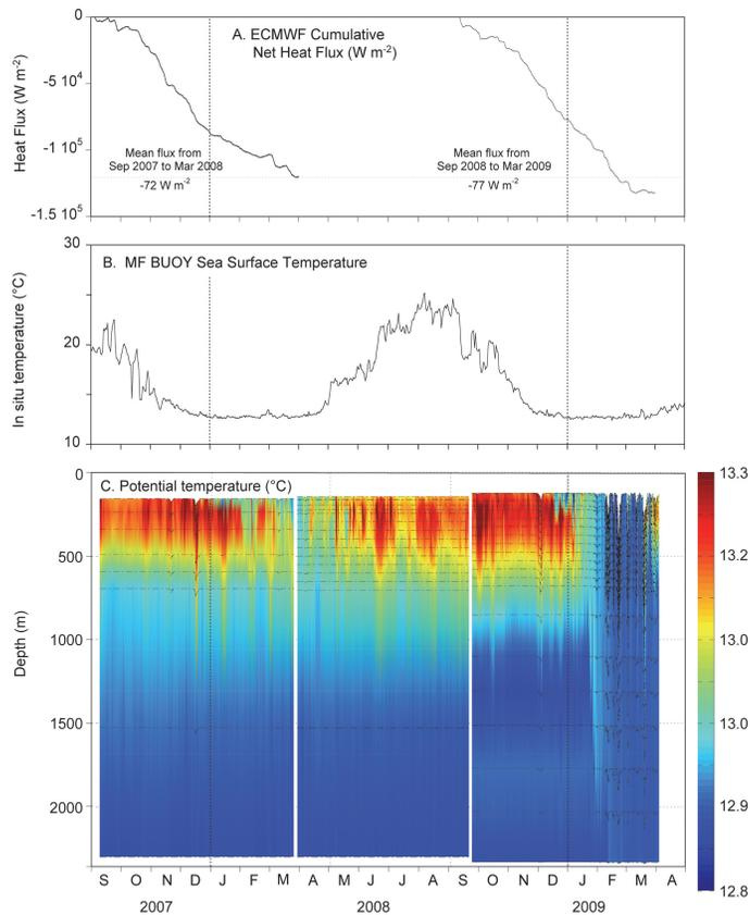
**Fig. 4.** Time-series of **(A)** surface cumulative net heat losses, **(B)** sea surface temperature measured at the Météo-France buoy in the convection area, and **(C)** vertical distribution of potential temperature at the SC2350 site from September 2007 to April 2009. Black dotted lines indicate the depth of the different temperature sensors. Note the deepening of the instruments during the winter 2008–2009 due to the strong currents.
