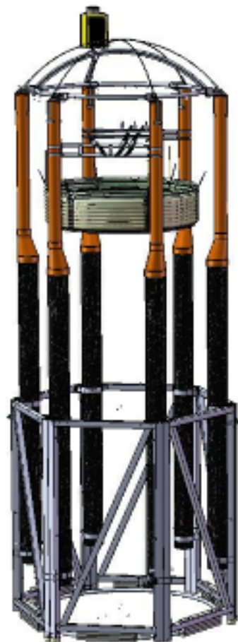
Fig. 1. Sketch of floatation frame with steel structure in grey, glass-fibre tubes in black and orange and up-folded enclosure bag in beige. Box on top represents flashlight with solar panels and radar reflector.
