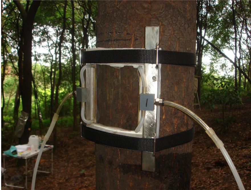
**Fig. 2.** Photograph of stem respiratory chamber.
