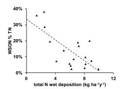
**Fig. 2.** Figure 2. Relationship between the proportion of Total N represented by WSON, and the wet deposition of total N at each site, showing the strong inverse relationship.
