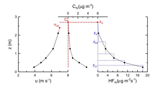
Fig. 1 Example profiles for wind speed, NH<sub>3</sub> concentration, and horizontal flux, HF<sub>N</sub>.
