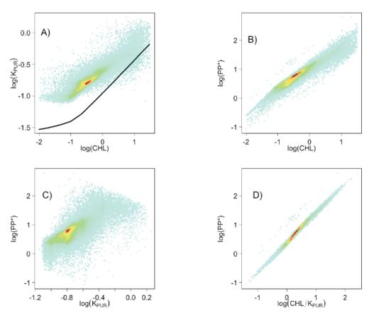
**Fig. 4.** Examples of relationships between (**A**) CHL and  $K_{PUR}$ , (**B**) CHL and PP normalized by surface PAR (PP\*), (**C**)  $K_{PUR}$  and PP\*, and (**D**) CHL/ $K_{PUR}$  and PP\* for the month of July 2007. The black line on panel (**A**) is  $K_{PUR}$  predicted from CHL using the empirical model of Morel and Maritorena (2001) for  $K_d$  and Matsuoka et al. (2011) for  $a_{ph}$ .
