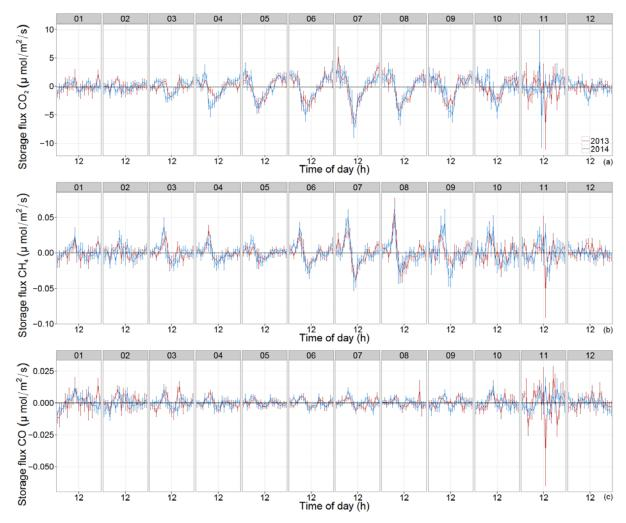
**Figure 6** Diurnal cycle of the storage flux estimates for CO<sub>2</sub> (a), CH<sub>4</sub> (b) and CO (c) for the years 2013 (red) and 2014 (blue).
