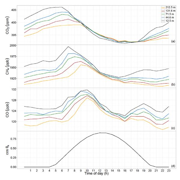
**Figure 4** Mean diurnal cycles of  $CO_2$  (a),  $CH_4$  (b), CO (c) in June for the sampling levels 12.5 m (black), 44.6 m (blue), 71.5 m (green) 131.6 m (red), and 212.5 m (yellow) together with the cosine of the solar zenith angle  $(\cos\theta_s)$  calculated for the geographical coordinates of site Beromünster.
