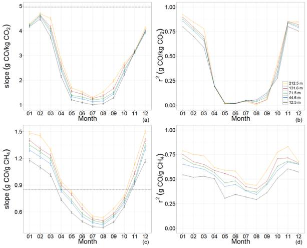
**Figure 2** Slope and  $r^2$  for  $\Delta \text{CO}/\Delta \text{CO}_2$  (a, b) and  $\Delta \text{CO}/\Delta \text{CH}_4$  (c, d) for the sampling levels 12.5 m (black), 44.6 m (blue), 71.5 m (green), 131.6 m (red) and 212.5 m (yellow). Horizontal dashed lines represent Swiss inventory estimates for 2013.
