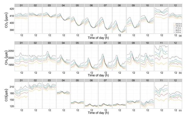
**Figure 3** Monthly mean diurnal cycles of CO<sub>2</sub>(a), CH<sub>4</sub> (b) and CO (c) for the sampling levels 12.5 m (black), 44.6 m (blue), 71.5 m (green) 131.6 m (red), and 212.5 m (yellow). The x axis on each subplot is centered at noon (UTC 12:00).
