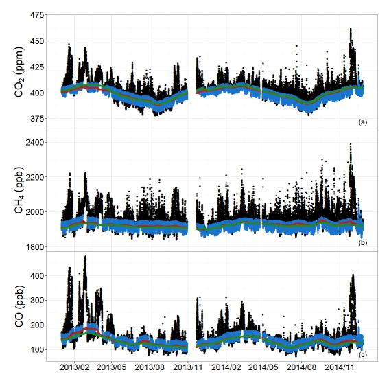
**Figure 1** Time series (December 2012-December 2014) of  $CO_2(a)$ ,  $CH_4(b)$ , and CO(c) at Beromünster for air sampled at 212.5 m. Color codes indicate: all measurements (black), estimated background values using  $2-\sigma$  filter (blue), moving average of 30 days based on the background estimates (red), and seasonal variations estimated by REBS (green).
