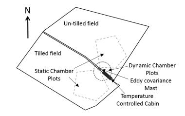
Figure 1 N<sub>2</sub>O fluxes were measured from two adjacent grassland fields at the Easter Bush Farm (Penicuik, Scotland). The north field remained un-tilled, while the south field was ploughed on the 1<sup>st</sup> of May 2012. An eddy covariance mast was setup next to a permanent cabin positioned between the fields. Dynamic chamber measurements were made within a 30 m radius of the cabin. Static chambers were spread out within the fetch of the eddy covariance mast.
