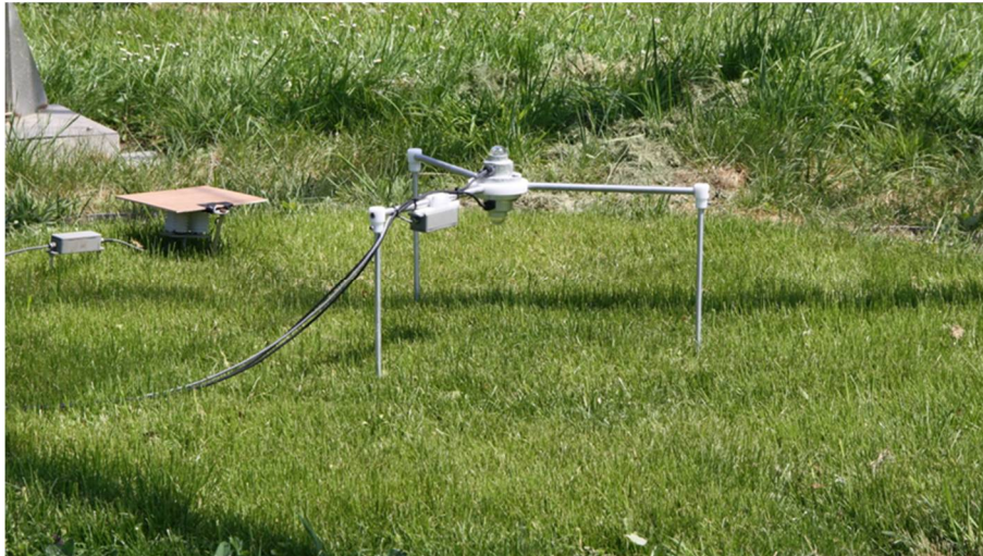
Figure S1: Homogeneous grass stand equipped with two pyranometers (upward and downward, for each hemisphere), a non-contact infrared thermometer for canopy temperature and a combined air temperature and relative air humidity sensor shielded by wooden panel.
