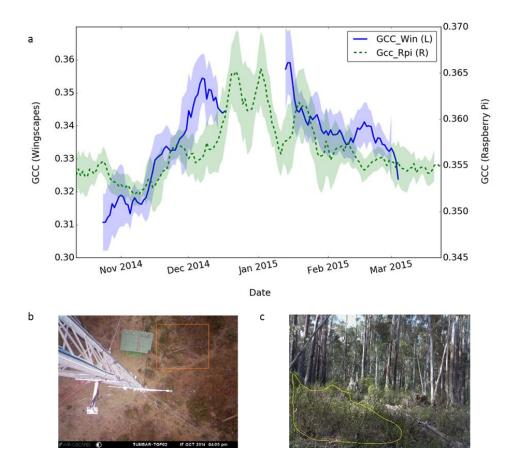
Figure 5: Phenocams in use at Tumbarumba (AU-Tum), New South Wales, Australia showing a) green chromatic coordinates (GCC) for understory vegetation from b) a downward facing wingscapes phenocam (region of interest inset) and an oblique facing raspberry pi (Rpi) phenocam (region of interest inset). GCC data are shown by an 8-day centred running mean with  $\pm$  90 % confidence shading.
